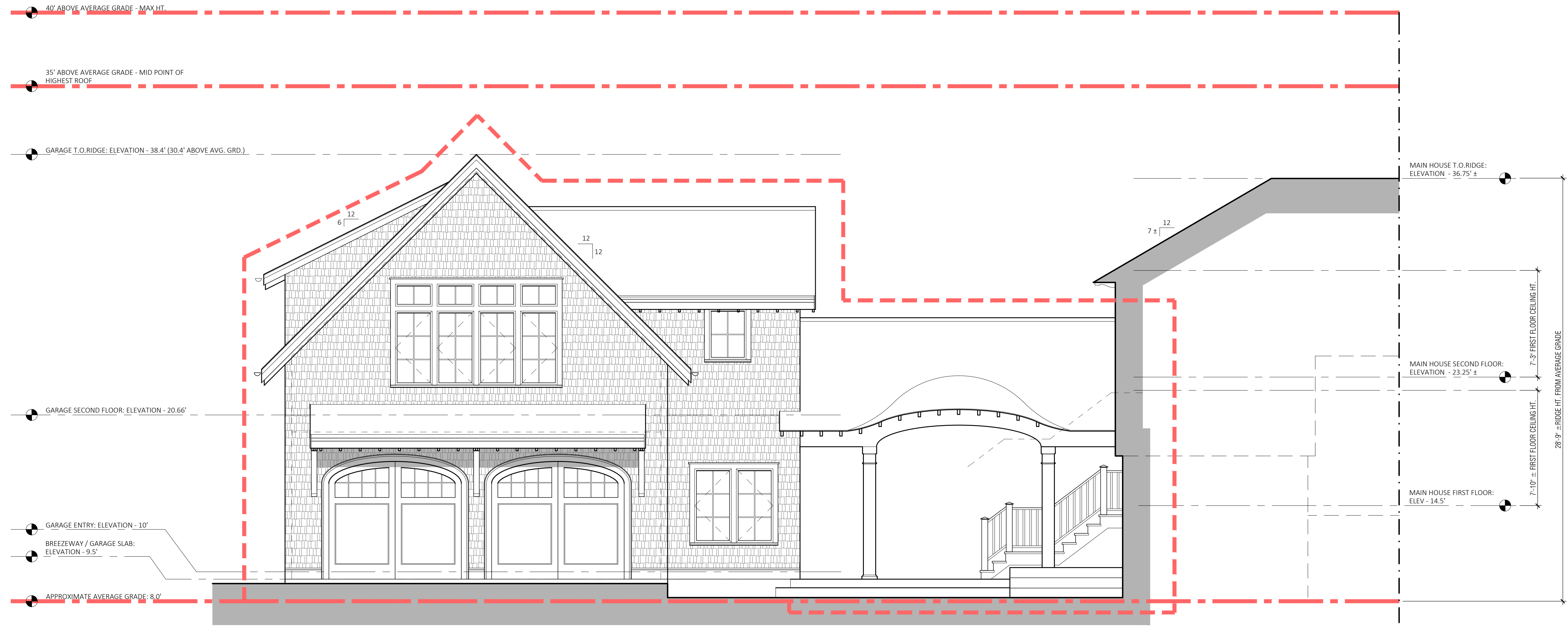
GARAGE & BREEZEWAY FRONT ELEVATION SCALE: 1/4" = 1'-0"
